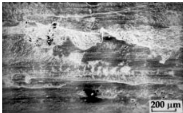
Fig. 9 Wear surfaces of the Cu-base alloy. (a) Tested at 0.42 m/s at the applied pressure of 1.0 MPa. (b) Tested at 0.42 m/s at the applied pressure of 12.0 MPa. (c) Tested at 4.62 m/s at the applied pressure of 1.0 MPa
