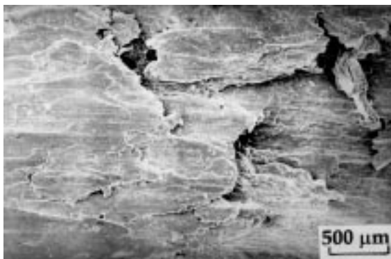
Fig. 8 Wear surfaces of the Zn-base matrix alloy. (a) Tested at 0.42 m/s at the applied pressure of 1.0 MPa. (b) Tested at 0.42 m/s at the applied pressure of 10.0 MPa. (c) Tested at 4.62 m/s at the applied pressure of 1.0 MPa. (d) Tested at 4.62 m/s at the applied pressure of 2.0 MPa. Arrow, sticking of debris
